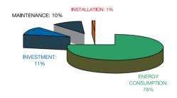
After 5 years of continuous compressor operation, the energy costs represent around 78% of the total cost of owership. By saving energy, the overall costs can be reduced considerably.
