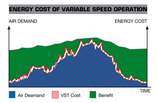
EKO - VST compressors are driven by a frequency converter. Factory air demand is measured continuously and the motor speed is automatically adjusted accordingly. Thus, the compressor produces compressed air by using only as much energy as needed, avoiding unnecessary waste.
