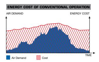
Standard compressors run with load - unload mode between two pressure points. When the pressure reaches the maximum level, the compressor goes unload. During the unload time, the compressor does not produce air; however it consumes about %30 of nominal power
